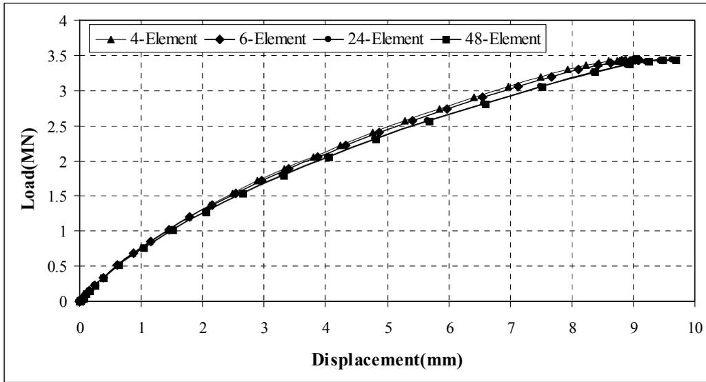
Figure 5. Load-Displacement Curves for Different Number of Elements
