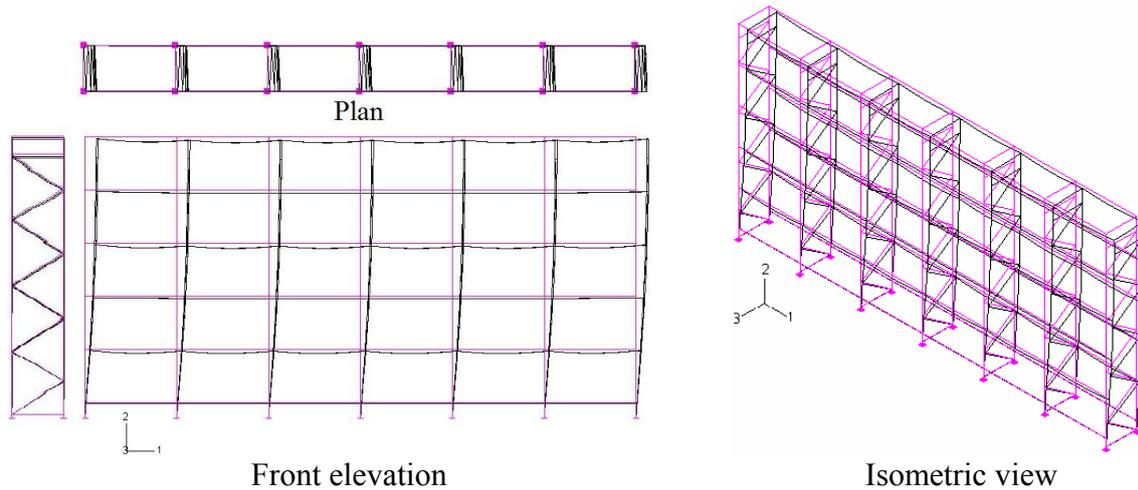
Figure 12. Collapse Mode for Case 7 (Semi-rigid Base-plate Frame)
