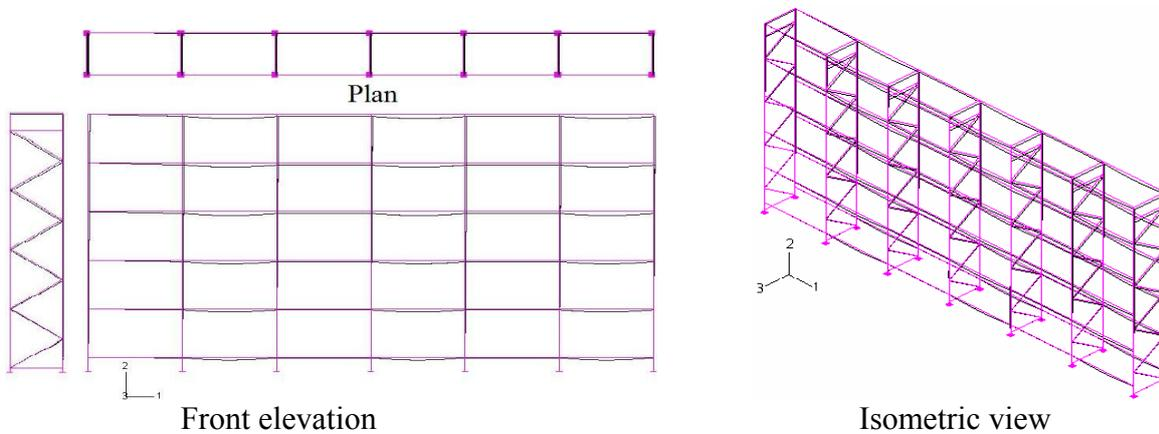
Figure 9. Collapse Mode for Case 2 (Semi-rigid Base-plate Frame)
