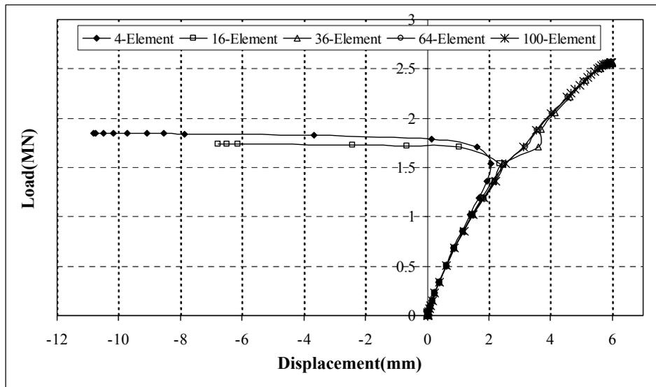
Figure 6. Load-Displacement Curves for Different Numbers of Elements
